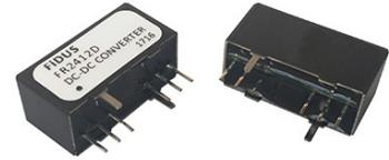
The FR series of power dense DC/DC converters come in both single and dual outputs in a SIP 8 pin package. Inputs are available in 24 & 48V versions with a 4:1 range and outputs from 3.3 to 24V single and dual  $\pm 5V$  to  $\pm 15V$ . The units operate from  $-40$  to  $+85^{\circ}C$  and come complete with remote on/off functionality. All models have a FIDUS 5 year warranty.
