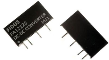
The FA series of low cost DC/DC converters come in both single and dual outputs in either a SIP 7 pin or DIP 14 pin package. Inputs are available in 5, 12, & 24V versions and outputs from 3.3 to 24V single and dual. The units operate from -40 to +85°C. High volumes are held in stock for the popular models. All models have a FiDUS 5 year warranty.
