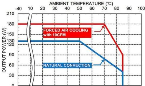
Derating Curve vs. Ambient Temperature
