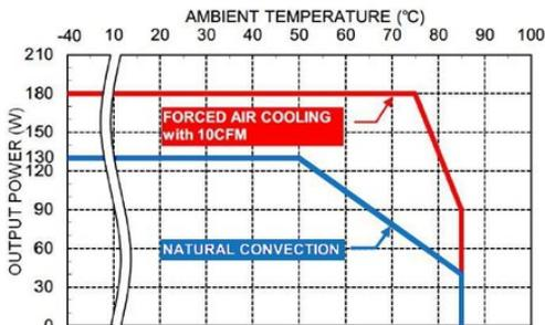
Derating Curve vs. Ambient Temperature
