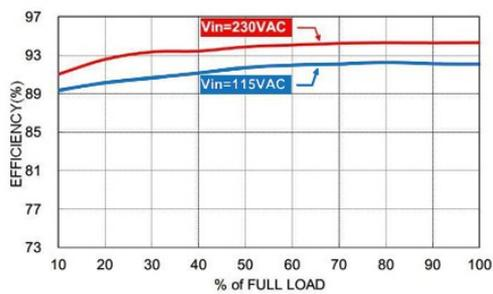
Efficiency vs. Output Load
