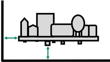
On installation customers must consider the required creepage and clearance distances between the PSU and the end-equipment enclosure. These distances vary depending on the installation class and safety standard requirements.
