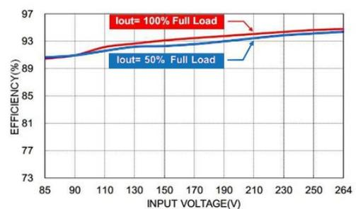
Efficiency vs. Input Voltage
