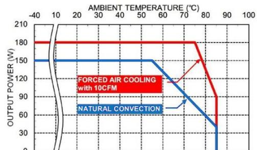
Derating Curve vs. Ambient Temperature
