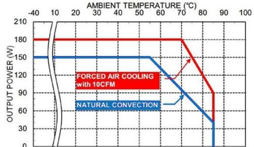
Derating Curve vs. Ambient Temperature
