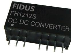
The FH series of low cost DC/DC converters come in both single and dual outputs in either a SIP 8 pin or DIP 16 pin package. Inputs are available in 5, 12, 24 & 48V versions and outputs from 3.3 to 24V single and dual. The units operate from -40 to +85°C. Traco TMR equivalent option. All models have a Fidus 3 year warranty.
