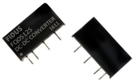
The FQ series of low cost DC/DC converters come in both single and dual outputs in either a SIP 7 pin or DIP 14 pin package. Inputs are available in 5, 12 & 24V versions and outputs from 3.3 to 24V single and dual. The units operate from -40 to +85°C. High volumes are held in stock for the popular models. All models have a FIDUS 3 year warranty.
