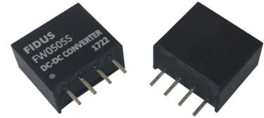
The FW series of low cost DC/DC converters come in single output in either a SIP 4 pin or DIP 8 pin package. Inputs are available in 3.3, 5, 12, 15, 24 & 48V versions and outputs from 3.3 to 24V. The units operate from -40 to +85°C. All models have a FiDUS 3 year warranty.
