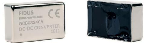
The GCB03 series of low cost DC/DC converters come in both single and dual outputs in a DIP 24 pin package. Inputs are available in 12, 24 & 48V versions with 2:1 range and outputs from 3.3 to 24V single and dual. The units operate from -40 to +85°C. High volumes are held in stock for the popular models. All models have a FiDUS 3 year warranty.
