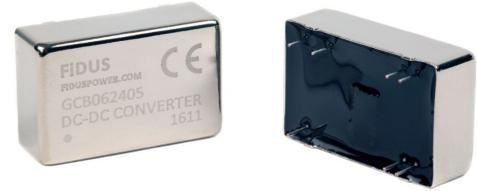
The GCB06 series of low cost DC/DC converters come in both single and dual outputs in a DIP 24 pin package. Inputs are available in 12, 24 & 48V versions with a 2:1 range and outputs from 3.3 to 24V single and dual. The units operate from -40 to +85°C. High volumes are held in stock for the popular models. All models have a FIDUS 3 year warranty.
