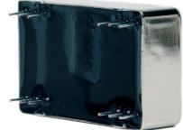
The GCP06 series of low cost DC/DC converters come in both single and dual outputs in a DIP 24 pin package. Inputs are available in 12, 24 & 48V versions and outputs from 3.3 to 24V single and dual. The units operate from -40 to +85°C. High volumes are held in stock for the popular models. All models have a Fidus 5 year warranty.
