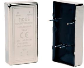
The HCA10 series of low cost DC/DC converters comes in both single and dual outputs. Inputs are available in 12, 24 & 48V versions with 2:1 range and outputs from 3.3 to 24V single and dual. The units operate from -40 to +85°C. 1500VDC isolation as standard with up to 3500VDC available (-H model). All models have a FiDUS 3 year warranty.
