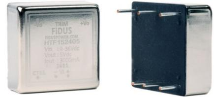
The HTF15 series of power dense DC/DC converters come in both single and dual outputs. Inputs are available in nominal 24 & 48V with 4:1 range and outputs from 3.3 to 15V single and dual. Remote on/off is available as an option. The units operate from -40 to +85°C. High volumes are held in stock for the popular models. All models have a FIDUS 3 year warranty.
