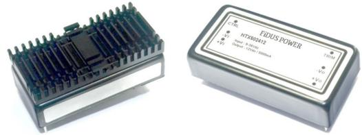
The HTX60 series of high power dense DC/DC converters come in both single and dual outputs. Inputs are available in 24 & 48V versions with 4:1 range and outputs from 5 to 15V single and dual. The DC/DC converters are very high efficiency of up to 93%, come complete with remote on/off and 10% trim as standard. The units operate from -40 to +100°C. All models have a FiDUS 3 year warranty.
