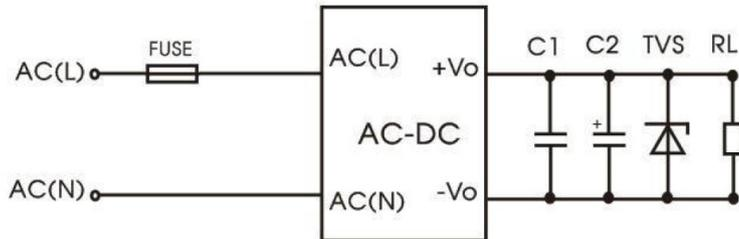
1. For a typical application we recommend placing these additional components close to the converter
