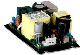
The AFR130 series of power dense, open frame AC-DC power modules offer 130W fan and 119-125W convection cooled in a 2.15 x 3.59" package. They have low no load (<0.3W) power consumption and excellent efficiency up to 91%. They have a wide operating temperature of -30 to 70°C and are available in output models of 12, 24 & 48V. All come with a FiDUS 3 year warranty.
