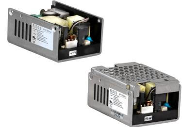
The AFR130-U/C series of power dense, conduction cooled, open frame AC-DC power modules offer 130W fan / conduction and 119-125W convection cooled in a 2.35 x 3.15" package. They have low no load (<0.3W) power consumption and excellent efficiency up to 91%. They have a wide operating temperature of -30 to 80°C and are available in output models of 12, 24 & 48V. All come with a FiDUS 3 year warranty.
