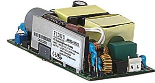
The AFR240 series of power dense, open frame AC-DC power modules offer 240W fan cooled in a 2x4" package. They have low no load (<0.5W) power consumption and excellent efficiency up to 94%. They have a wide operating temperature of -30 to 80°C and are available in output models of 12, 24 & 48V. All come with a FIDUS 3 year warranty.
