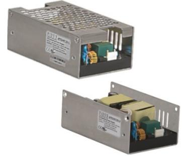
The AFR240U/C series of power dense, U-channel or covered AC-DC power supplies offer 240W convection cooled in a 2.44 x 4.1" package. They have low no load (<0.5W) power consumption and excellent efficiency up to 94%. They have a wide operating temperature of -30 to 80°C and are available in output models from 12, 24 & 48V. All come with a Fidus 3 year warranty.
