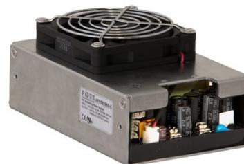
The AFR500C series of power dense, open frame AC-DC power modules offer 500W in a 3.25 x 5.11" package. They have excellent efficiency up to 91.5%, remote on off, 5V stand by, DC OK, remote sense, a wide operating temperature of -30 to 80°C and are available in output models 12, 24 & 48V. All come with a Fidus 3 year warranty.
