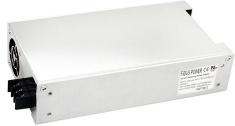
The VQF700 series of compact enclosed AC-DC PSUs that provide 600-700W from a fan cooled 3.66 x 7.16" package. The range is approved for use in both IT and industrial applications and is available in a range of 12 to 48V output. The units are fully featured with 5V standby rail, remote on/off, power good signal and remote sense. All with a FIDUS 3 year warranty.
