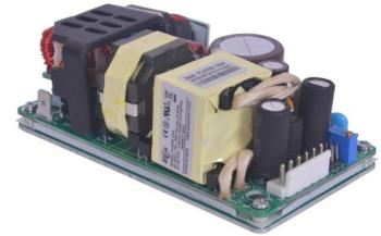
The FLS250 series of power dense open frame AC-DC power modules offer up to 250W convection cooled and 350W fan cooled in a 2 x 4" or 3 x 5" mount. The 1.5" low profile product is available with JST or screw terminal output and offers an onboard 12V fan output and optional 5V 0.5A stand by, remote on off and current share for parallel operation. All come with a 2 year warranty.
