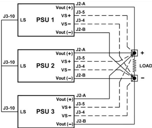
The volt sense lines must all be connected to one point and the output voltage of each the power supplies must be adjusted to be within 1% for the current share to operate. Should they not be adjusted the current share will not function. When using the load share function derate the cumulative power total by 10%. Please follow the below step by step process to ensure smooth operation:
