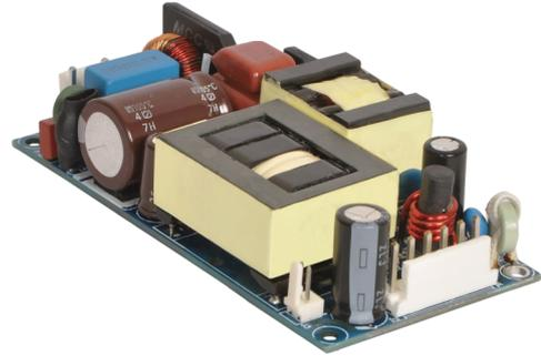
The WLP225 series of low profile, open frame AC-DC power modules offer 120W convection cooled and 225W fan cooled in a 4" x 2" package. The 1" low profile product is available with molex or screw cage terminals and offers an onboard fan output (12V 0.5A). They are chassis mount, low noise, low no load (<0.5W), with a wide operating temperature of -40 to 70°C, in a range of voltages from 12V to 58V and all come with a FIDUS 2 year warranty.
