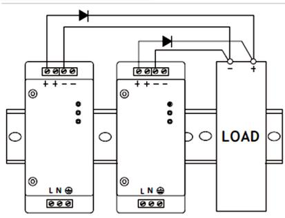
Parallel operation is possible as per drawing. Only identical units can be used in this way. Do not mix powers or voltages.
