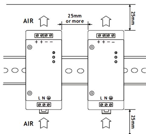
For best thermal performance allow for ventilation either side of the unit to neighbouring power supply units and above and below the unit as per diagram. Spacing can be reduced with forced air cooling.
