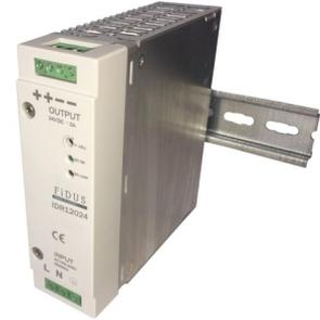
The IDR120 series of DIN rail power supplies provide 120W of power in a slim 40mm package. The units are fully featured with built in EMI filter and over voltage, over current and short circuit protections. Outputs available; 12, 24 or 48V and every unit comes with a FIDUS 3 year warranty.
