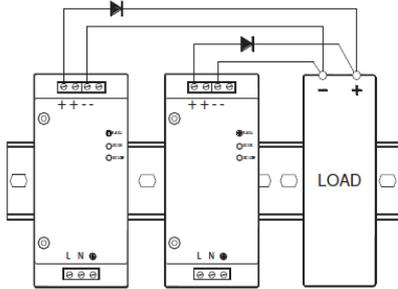
Parallel operation is possible as per drawing. Only identical units can be used in this way. Do not mix powers or voltages.
