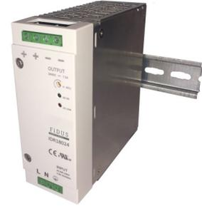
The IDR180 series of DIN rail power supplies provide 180W of power in a slim 50mm package. The units are fully featured with built in EMI filter and over voltage, over current and short circuit protections. Outputs available; 24 or 48V and every unit comes with a FiDUS 5 year warranty.
