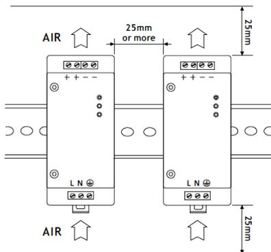
For best thermal performance allow for ventilation either side of the unit to neighbouring power supply units and above and below the unit as per diagram. Spacing can be reduced with forced air cooling.
