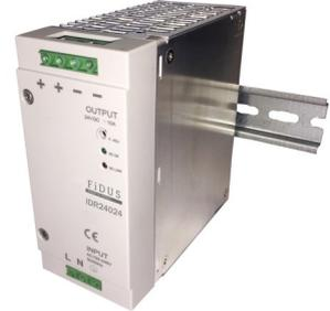
The IDR240 series of DIN rail power supplies provide 240W of power in a slim 60mm package. The units are fully featured with built in EMI filter and over voltage, over current and short circuit protections. Outputs available; 24 or 48V and every unit comes with a FIDUS 3 year warranty.
