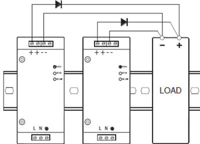
Parallel operation is possible as per drawing. Only identical units can be used in this way. Do not mix powers or voltages.
