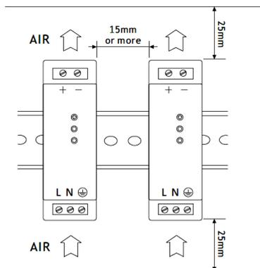
For best thermal performance allow for ventilation either side of the unit to neighbouring power supply units and above and below the unit as per diagram. Spacing can be reduced with forced air cooling.
