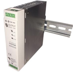
The IDR50 series of DIN rail power supplies provide 50W of power in a slim 30mm package. The units are fully featured with built in EMI filter and over voltage, over current and short circuit protections. Outputs available; 12, 24 or 48V and every unit comes with a FiDUS 3 year warranty.
