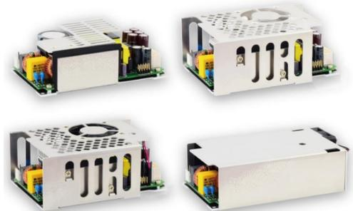
The MAH450 series of compact open frame AC-DC PSUs provide 320W convection, 350W conduction and 450W fan cooled power from a 3" x 5" package. The range is approved for use in both IT and medical applications and is available in 12-53V units. The units are fully featured with power good, remote on off and voltage adjust. They are available in four variants; open frame, enclosed, top fan and end fan. All units come with a FiDUS 5 year warranty.
