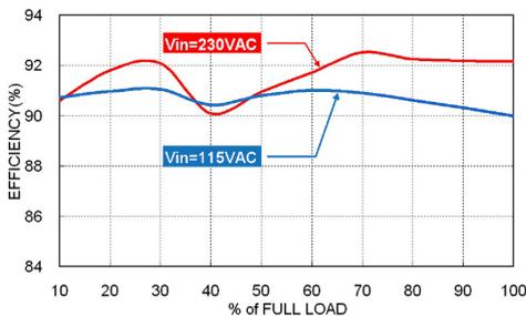
TAD125US24B Efficiency vs. Output Load
