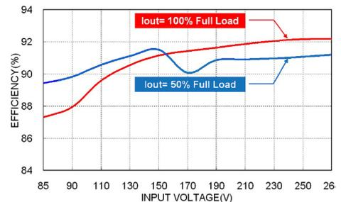
TAD125US24B Efficiency vs. Input Voltage
