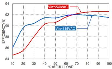
TAD50US12 Efficiency VS Output Load
