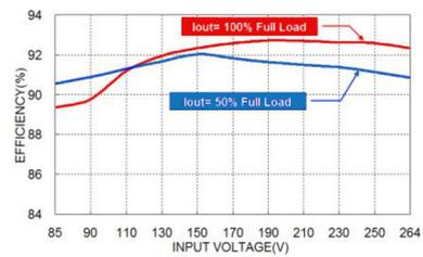
TAD50US12 Efficiency vs. Input Voltage
