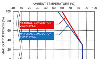
Derating Curve vs. Ambient Temperature
