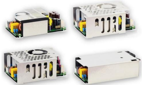
The TAH450 series of compact open frame AC-DC PSUs provide 320W convection, 350W conduction and 450W fan cooled power from a 3" x 5" package. The range is approved for use in Industrial and IT applications and is available in 12-53V units. The units are fully featured with power good, remote on off and voltage adjust. They are available in four variants; open frame, enclosed, top fan and end fan. All units come with a Fidus 3 year warranty.
