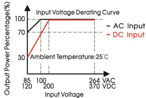
Note: 1. With an AC input voltage between 85 - 100VAC and a DC input between 120 - 200VDC the output power must be derated as per the temperature derating curves;
