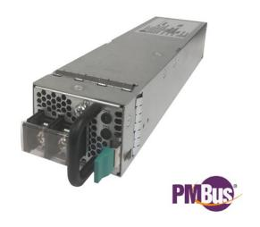
The MPR0712DC series provides high efficiency isolated power from the DC input mains. The industry standard PMBus® compliant I2C communications bus offers a full range of control and monitoring capabilities. The SMBAlert signal pin automatically alerts customers of any state change within the power supply.
