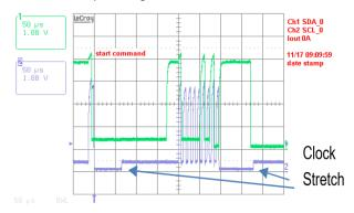
**1<sup>2</sup>C Bus Lock-Up detection:** The device will abort any transaction and drop off the bus if it detects the bus being held low for more than 35ms.
