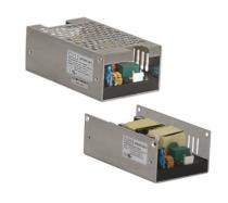
The AFR240U/C series of power dense, U-channel or covered AC-DC power supplies offer 240W convection cooled in a 2.44 x 4.1" package. They have low no load (<0.5W) power consumption and excellent efficiency up to 94%. They have a wide operating temperature of –30 to 80°C and are available in output models from 12, 24 & 48V. All come with a Fidus 3 year warranty.
