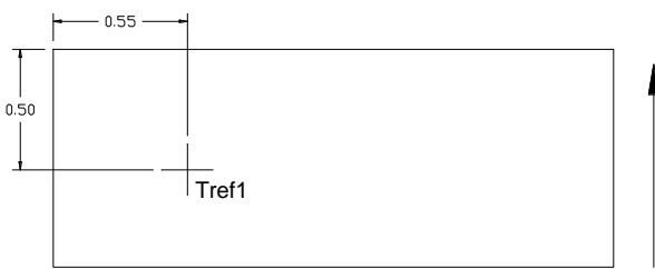
Figure 18. Case ( T_{REF} ) Temperature Measurement Location (top view).
