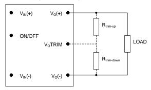
Figure 11. Circuit Configuration to Trim Output Voltage.
