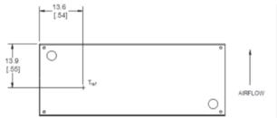
Figure 12.  $T_{\text{ref}}$  Temperature Measurement Location for Module with Heatplate.
