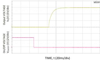
Figure 4. Typical Start-up Using Remote On/Off, negative logic version shown ( $V_{IN}$  = 48V,  $I_0$  =  $I_{O,max}$ ).
