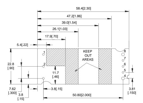
**TH Recommended Pad Layout (Component Side View)**
