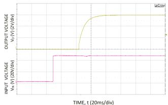
Figure 5. Typical Start-up Using Input Voltage ( $V_{IN} = 48V$ ,  $I_0 = I_{O,max}$ ).
