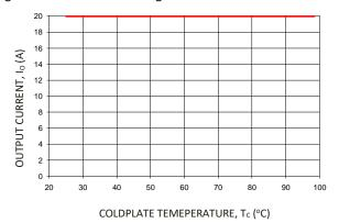
Figure 15. Derated Output Current versus Cold Wall Temperature with local ambient temperature around module at 75°C;  $V_{\text{IN}}$  =48V.
