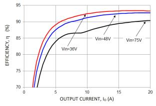
Figure 1. Converter Efficiency versus Output Current.
