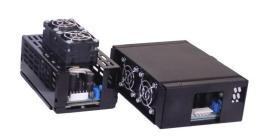
The FLS400 series of power dense chassis mount AC-DC power modules offer a power dense 400W in two mechanical formats, depending on your power envelope. They have a high power density of 23.7W/inch<sup>3</sup> and are available in 6 output voltages from 12-58V (custom voltages possible) with an adjustment of 3% and optional current share card for parallel operation. All come with a FiDUS 5 year
