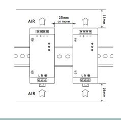
For best thermal performance allow for ventilation either side of the unit to neighbouring power supply units and above and below the unit as per diagram. Spacing can be reduced with forced air cooling.
