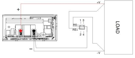
Remote sensing function wiring diagram
