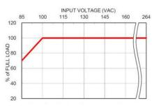
Derating Curve vs. Input Voltage MAF300
