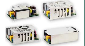
The MAH450 series of compact open frame AC-DC PSUs provide 320W convection, 350W conduction and 450W fan cooled power from a 3" x 5" package. The range is approved for use in both IT and medical applications and is available in 12-53V units. The units are fully featured with power good, remote on off and voltage adjust. They are available in four variants; open frame, enclosed, top fan and end fan. All units come with a FiDUS 5 year warranty.
