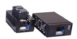
The MFLS400 series of power dense chassis mount AC-DC power modules offer a power dense 400W in two mechanical formats, depending on your power envelope. They have a high power density of 23.7w/inch<sup>3</sup> and are available in 6 output voltages from 12-58V (custom voltages possible) with an adjustment of 3% and optional current share card for parallel operation. All come with a Fidus 3 year
