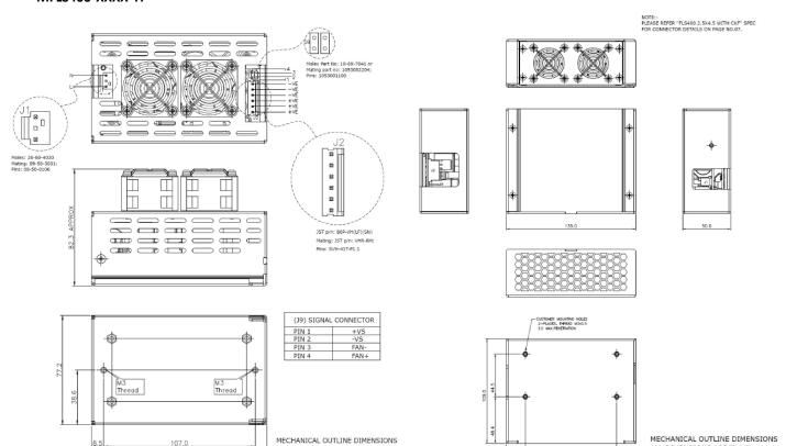
ALL DIMENSIONS ARE IN MM GEN.TOLERANCE:+/-0.5 MM
