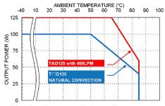
Derating Curve vs. Ambient Temperature Vin=230VAC
