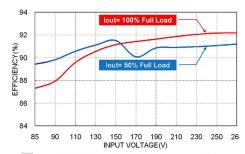
T□D125US24B Efficiency vs. Input Voltage
