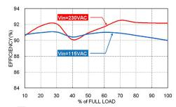
T□D125US24B Efficiency vs. Output Load
