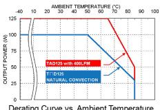
Derating Curve vs. Ambient Temperature Vin=115VAC
