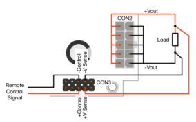
(a) Sense pins connect to corresponding polarity of Vout pin
