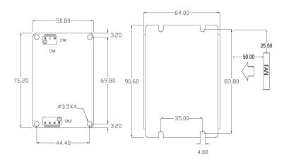
3. CN2: Output header: JST B4P-VH-B pitch: 3.96mm mating part: JST VHR-4N
