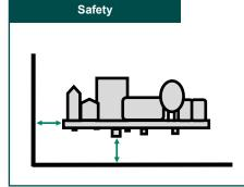
On installation customers must consider the required creepage and clearance distances between the PSU and the end-equipment enclosure. These distances vary depending on the installation class and safety standard requirements.
