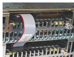
Shelf-to-shelf cable connection (part # CC848848952)
