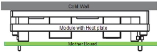
**Figure 14. Cold Wall Mounting**
