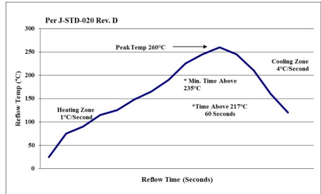
**Figure 19. Recommended linear reflow profile using Sn/Ag/Cu solder.**
