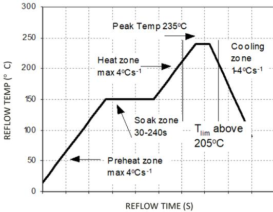
**Figure 17. Reflow Profile for Tin/Lead (Sn/Pb) process.**
