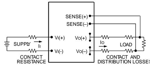
Figure 10. Circuit Configuration for remote sense .
