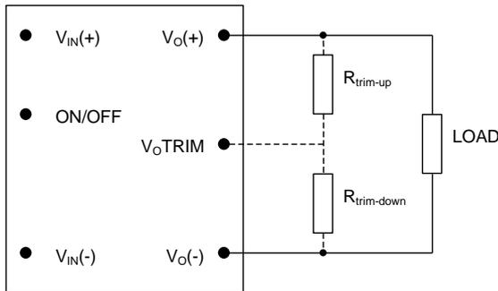
**Figure 11. Circuit Configuration to Trim Output Voltage.**
