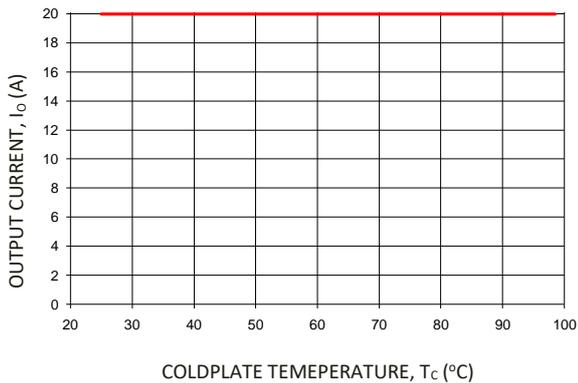
**Figure 15. Derated Output Current versus Cold Wall Temperature with local ambient temperature around module at 75°C; V<sub>IN</sub> =48V.**
