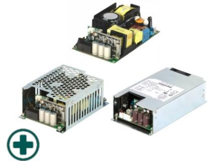
The MAC450 series of open frame power dense AC-DC power modules offer 250W convection and 450W of power with fan cooling in a 3 x 5" package. The units are designed for use in medical and ITE applications, are very efficient and have low emissions, meeting EN55011 Level B and 4th edition EMC immunity EN60601-1-2. They have an operating temperature range from -20 to +70°C operating from 85 to 264VAC. Outputs are available from 12 to 56V with 5V 1A stand by and 12V 0.6A fan rail.
